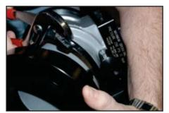
**Step #5)** Once the strip is exposed by several inches you may remove using pliers.
