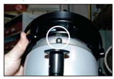
Step #9B) If desired, install lock out ball. Apply a small amount of grease to the ball pocket to help retain the ball in position. Push coupling on completely. If lock out ball is being used, note alignment.
