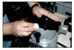
Step #12) Use a degreaser to clean the area of the port if the cover type is used. Use short end of the THA401 to assist in the installation of the port plug. Install till flush.
