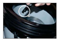
Step #10) Insert polymer ring into the port with the blunt end first.
