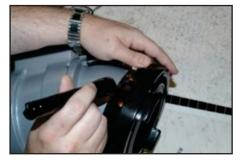
**Step #2)** If the coupling swivels, rotate till the end on the polymer ring can be seen through the access port. The ring can also be moved with the seal pick if required.
